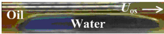
Fig. 12. A picture of an eccentric elongated water drop taken in an upward inclined glass by-pass line (I.D.=15 mm, V_w = 10 ml).
